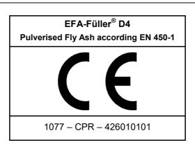
Type II addition for concrete according to EN 206-1
